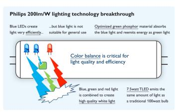
At the heart of the new TLED is the Philips Lumileds InGaN LED, recognized as the world's highest performing blue LED.
