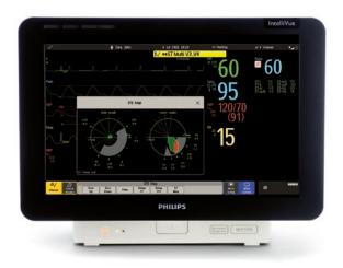
Whether you are examining the patient in a brightly lit environment or allowing the patient to rest with room lights dimmed, you won't have to adjust the monitor's display brightness. The display, with its ambient light sensor, automatically adjusts screen brightness to maintain readability in nearly any lighting environment.
