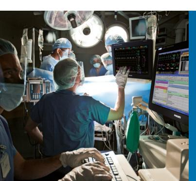
Ambient light adjustment is just part of why the IntelliVue MX550 is an excellent solution for critical care settings and the OR. In the OR, for example, the display automatically adapts to lights being dimmed or brightened during different stages of surgery, reducing overall light pollution.
