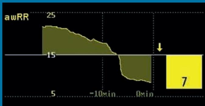
Example of Horizon Trend of respiration rate: The patient's airway respiratory rate is trending downwards at seven breaths per minute, under the target set at 15 breaths per minute.
