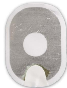
Figure 3: Gel almost completely separated from backing.
