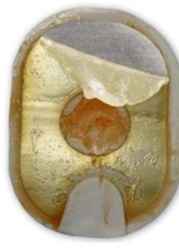
Figure 2: Separated, folded gel may also have a discolored and/or melted appearance.
