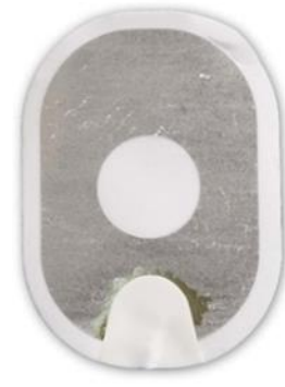
Figure 3: Gel almost completely separated from backing.
