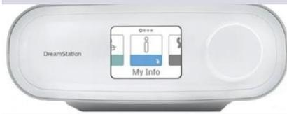
2.2 The display screen will illuminate and "My Info" will appear when successfully connected to AC Power
