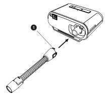
2. Press the heated tubing into place over the air outlet port until the tabs on the side of the tube click into place in the slots on the sides of the outlet port.
