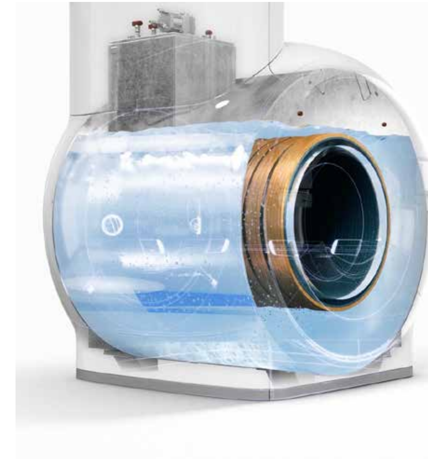
Classic magnet technology - ~1,500 liters of liquid helium
