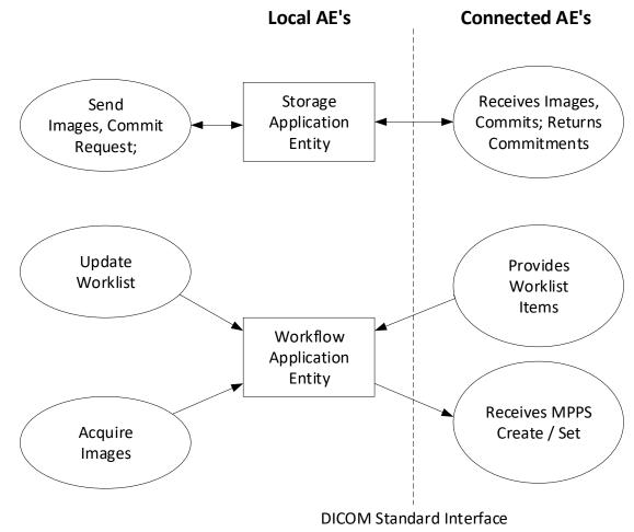
Figure 1 APPLICATION DATA FLOW DIAGRAM
