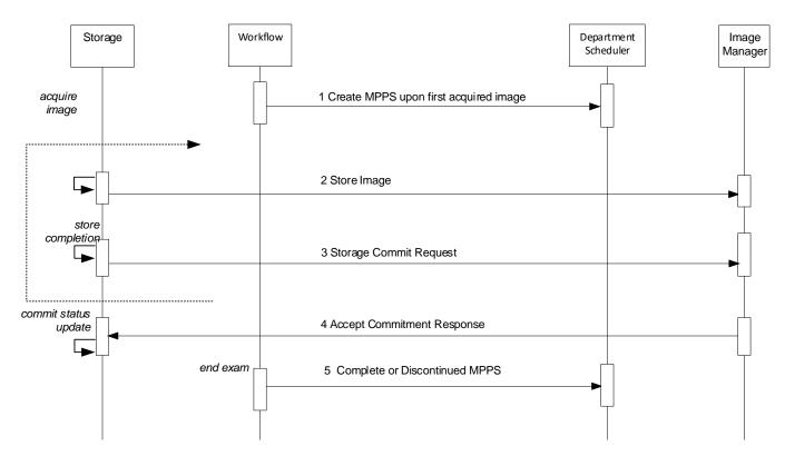
**Figure 2** Sequencing Constraints – Configured to Send as Images are Acquired
