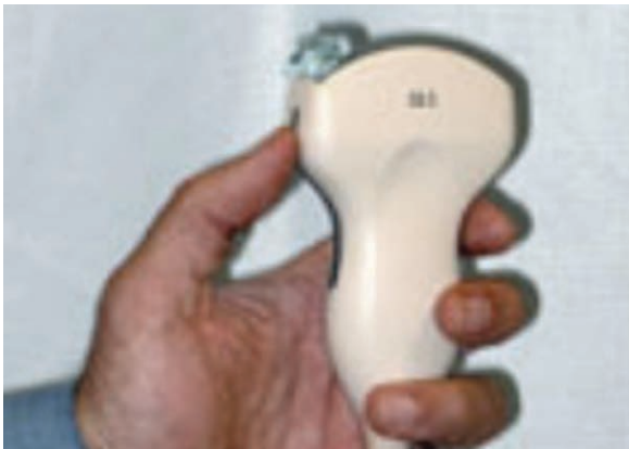
[Figure 1] Photo demonstrating small amount of gel on the side of the transducer corresponding to the orientation marker.
