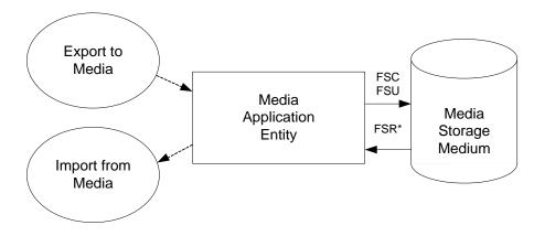
Figure 9 APPLICATION DATA FLOW DIAGRAM FOR MEDIA STORAGE
