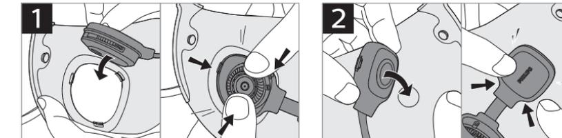
Press the electric fan into the fan ring from the inner side of the mask cover. Make sure that all 3 snaps on the ring are fastened.
