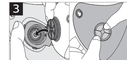
Press the filter exhalation valve tightly into the electric fan.
