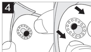
Match the filter's 8 shape buckle with the button on the inner side of the mask cover. Pull the filter until the button slips into the smaller side of the buckle.
