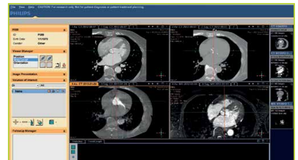
Multi-modal data evaluation for a TAVI case: CTA, native CT for calcium scoring, XperCT with LV-injection, whole heart MR
