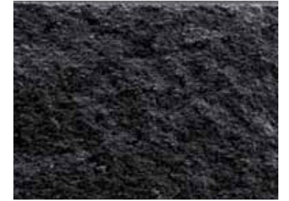
Alumina, pore size > 1µm SEM picture magnified x40
