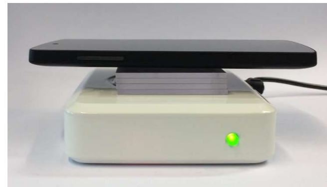
Nexus 5 charging on Royer demonstrator 15 mm coil to coil distance
