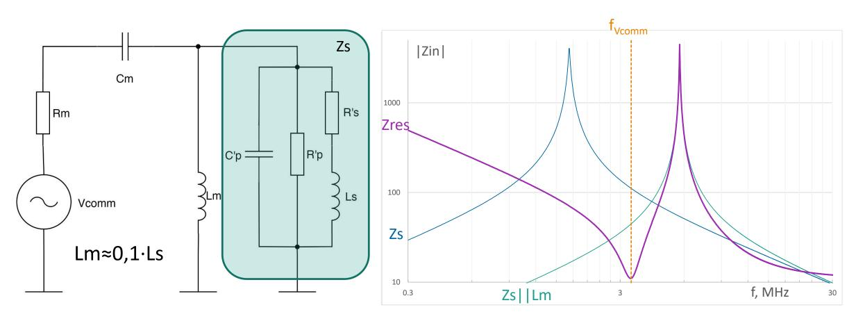
On the resonance frequency f<sub>Vcomm</sub> the parasitic parallel resonance is **moved in higher frequency region**
