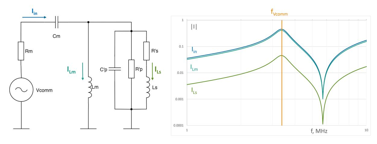
At the high-frequency resonant frequency, the resonant current divided between Ls and Lm impedance-wise.
