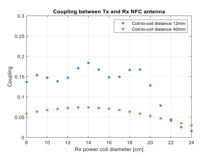
Sufficient coupling over the complete PRx diameter range with a PTx antenna of 21cm
