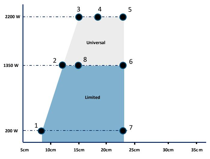
Test PRx power coil diameter
