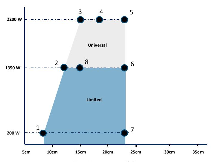
Test PRx power coil diameter
