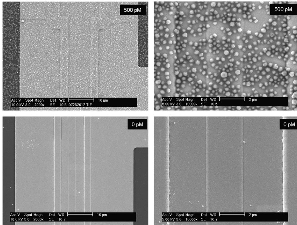
**Fig. 4.** SEM pictures of magnetic particles on the sensor after a one-step assay. In the upper images two different magnifications of one sensor are shown for a 500 pM PCR product. The GMR sensor is visible flanked by the current wires. The lower images were taken after a one-step assay with blank product (PCR without template).
