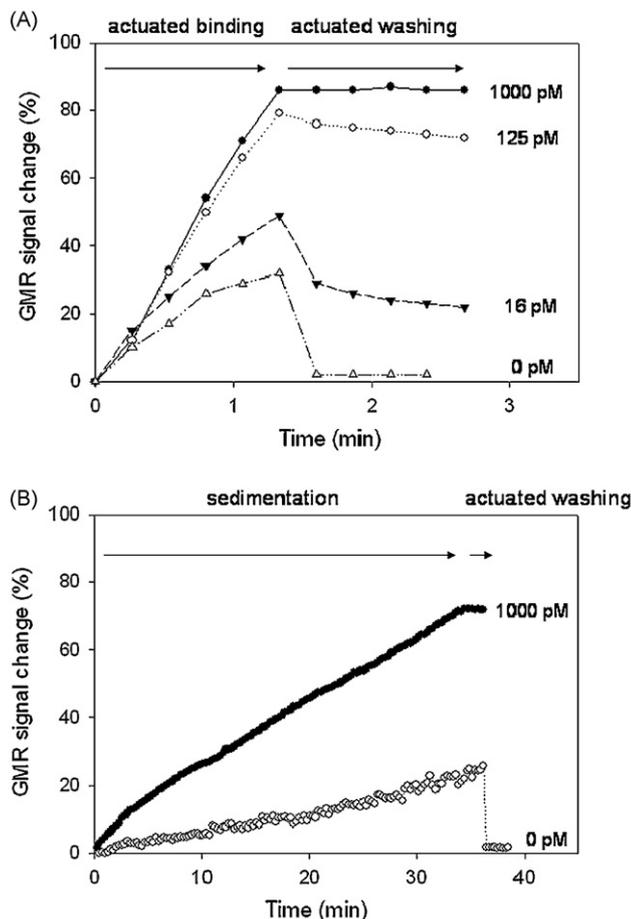
**Fig. 2.** Time trace of a one-step assay comparing (A) magnetic actuation with (B) sedimentation/diffusion of magnetic particles. At  $t = 0$  the sample and magnetic particles were injected. For 1000 pM *E. coli* PCR product, an actuated assay takes 1.5 min. The same signal is reached in more than 30 min in a sedimentation/diffusion assay.
