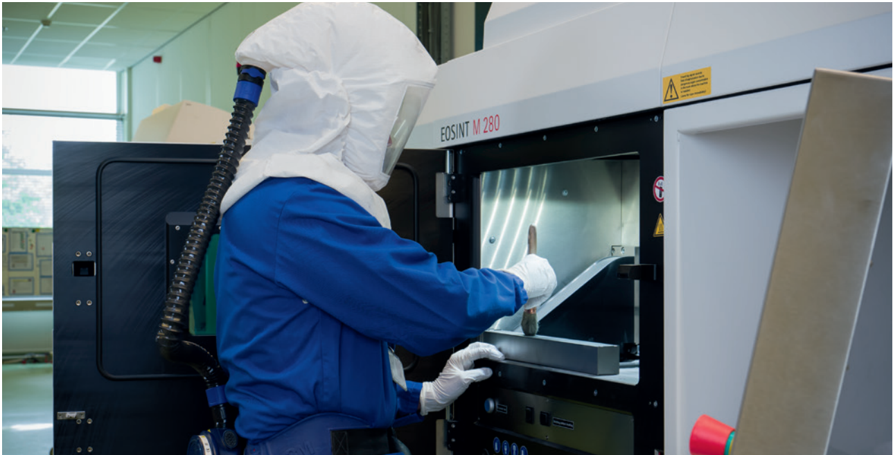
Removing and cleaning 3D-printed tungsten parts
