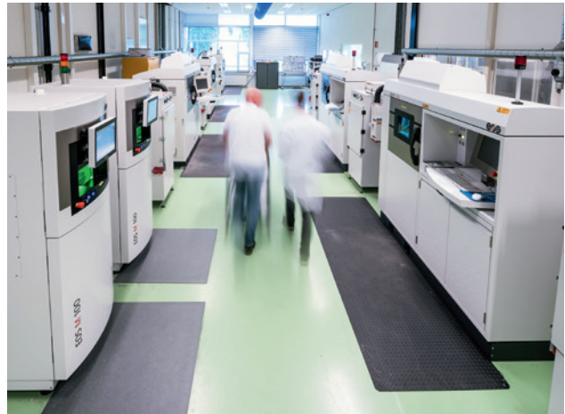
Figure 2: DMLS factory for mass-production of high-precision 3D-printed tungsten parts.
