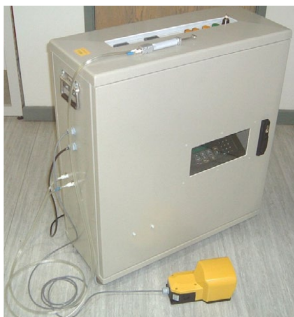
Initial experimental device used to carry out first clinical tests on safety and efficacy – a foot pedal activated single shots of high-velocity droplet sprays.
