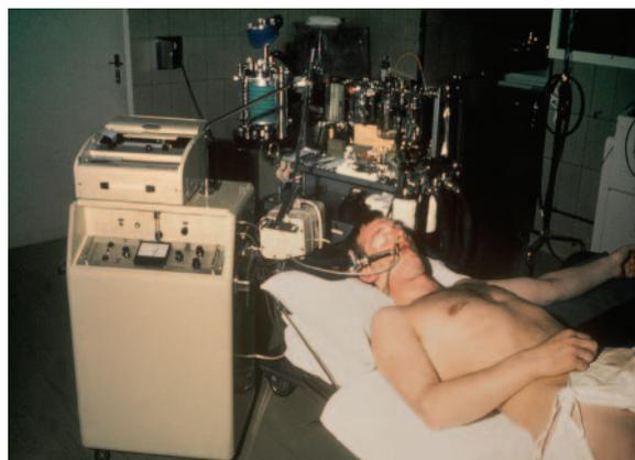
**Figure 3.** The first CO<sub>2</sub> analyzer (Godart Capnograph medical CO<sub>2</sub> analyzer) in the Central Military Hospital, Utrecht, The Netherlands (1962). On top is the one channel Omnicriptor. Photo: Lt. Klunder (Photo used with permission from Prof. Bob Smalhout).
