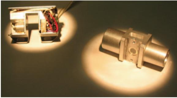
**Figure 12.** Original prototype Capnostat CO<sub>2</sub> sensor and airway adapter (Image courtesy of Respironics, Inc., Murrysville, PA.).
