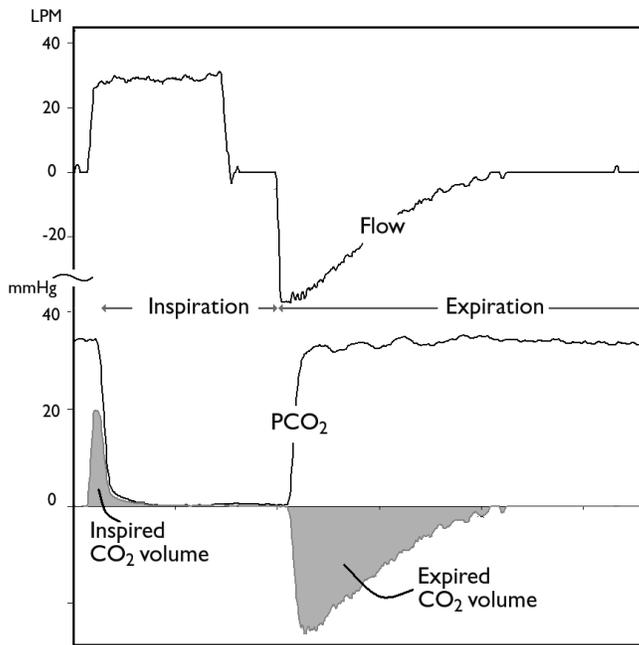
**Figure 1** - Plot of flow and CO<sub>2</sub> waveforms for an individual ventilator delivered breath with product showing inspired and expired CO<sub>2</sub> volumes. LPM: liters per minute.
