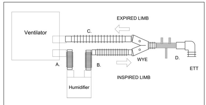
Figure 6 - Ventilator with breathing circuit with proximal mainstream flow sensor (grayed) and portion of sidestream gas sampling tube (grayed) shown.
