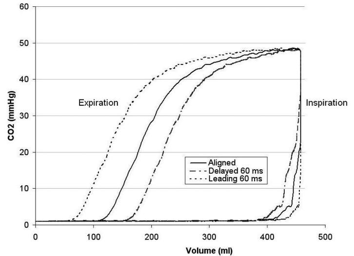
**Figure 2** - Volumetric Capnogram showing both expiratory and inspiratory limbs and illustrating the effect of time misalignment. Note if the CO<sub>2</sub> waveform is delayed relative to the volume, the loop gets smaller on both ends, conversely when the CO<sub>2</sub> waveform is advanced relative to volume, the loop gets larger on both ends.
