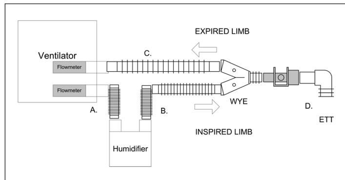
Figure 5 - Ventilator with breathing circuit with proximal mainstream CO<sub>2</sub> sensor (grayed) and flow sensors internal to ventilator (grayed).
