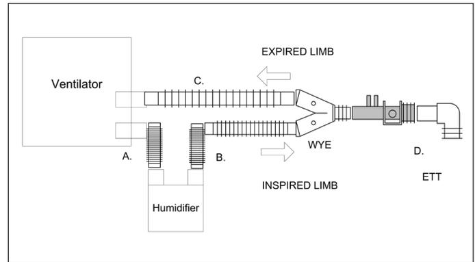
**Figure 3** - Ventilator with breathing circuit with humidifier on inspiratory limb with proximal mainstream combined  $\text{CO}_2$ /flow sensor (grayed). Conditions at A through D are described below:
