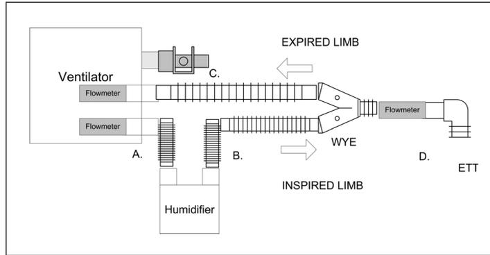
Figure 4 - Ventilator with breathing circuit with proximal mainstream flow sensor (grayed) and "mainstream" CO<sub>2</sub> sensor at exhalation port of ventilator (grayed).
